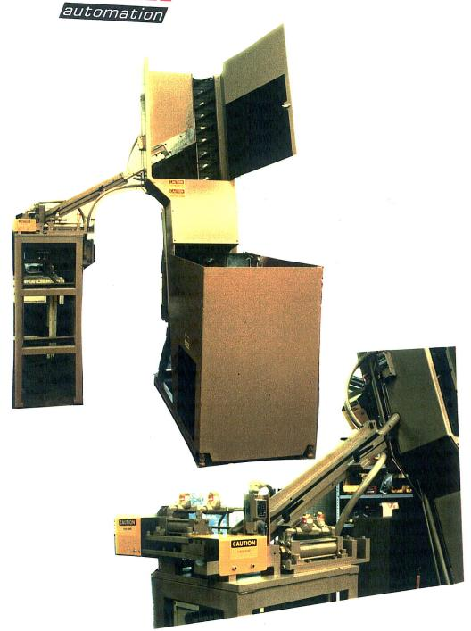
FEED FROM A RANDOM LOADED FLOOR MOUNTED HOPPER, STEEL BILLETS, 3/4 TO 1 1/4 DIA. X 3 TO 4" LG. THE BILLETS WILL BE ORIENTED END TO END THEN FED AND TRANSFERRED ROLLING ONE AT A TIME INTO A PUSHER, THEN ADVANCED TO A INDUCTION HEATER FOR FORGING AT A HEIGHT OF 55" ABOVE THE FLOOR AT A RATE OF 24 BILLETS PER, MIN. 7 1/2" WIDE ELEVATOR BELT, 12 CU. FT. HOPER. DWG. P 7674 R
