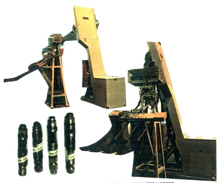
FEED FROM A RANDOM LOADED FLOOR MOUNTED HOPPER, POWER STEERING GEAR IN PUT SHAFTS. THE SHAFTS WILL BE FED END TO END THEN ORIENTED SMALL END LEADING THEN SHUTTLED IN TO FOUR STREAMS AND DISCHARGED AT A HEIGHT OF 42" ABOVE THE FLOOR, 8" APART AT A FEED RATE OF 640 TO 800 PER. HOUR. FEEDING A DIAL FOR A REAMER.
