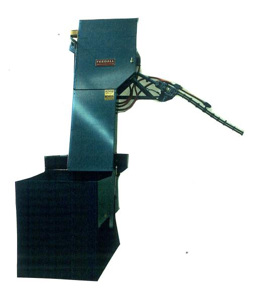
FEED FROM A RANDOM LOADED FLOOR MOUNTED HOPPER, PISTON PINS. THE PINS WILL BE ORIENTED END TO END THEN FED TO AN ESCAPEMENT THEN ESCAPED ONE AT A TIME COUNTED AND FED TO A POINT 65" ABOVE THE FLOOR AT A RATE OF 25 TO 35 PER. MIN.
