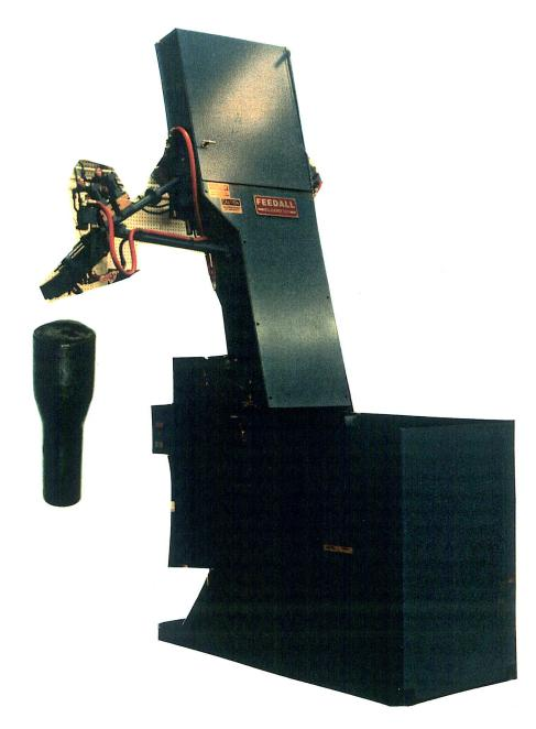
FEED FROM A RANDOM LOADED FLOOR MOUNTED HOPPER, STEERING PINION FORGINGS. THE PINIONS WILL BE ORIENTED END TO END THEN ESCAPED ONE AT A TIME HANGING IN TO A LOAD CHUTE OF A NEW BRITTON TURNING MACHINE AT A RATE OF 8 TO 12 PER. HOUR AT A HEIGHT OF 60" ABOVE THE FLOOR. 7 1/2" WIDE ELEVATOR BELT, 12 CU. FT. HOPPER.
