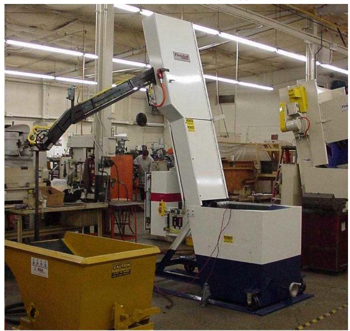
**APPLICATION:** Feed from a random loaded, floor mounted hopper, Universal Joint Spider Forgings.
