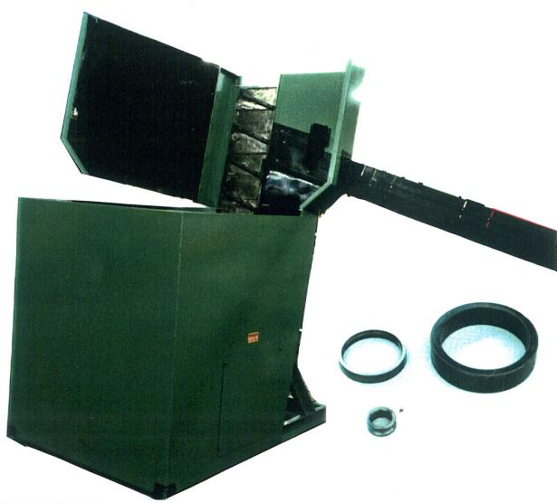
FEED FROM A RANDOM LOADED FLOOR MOUNTED HOPPER, BEARING RACES 1 T 6" DIA. X 1/4 TO 1 1/4" THICK. THE BEARINGS WILL BE ORIENTED DIAMETER TO DIAMETER ROLLING THEN FED TO A HEIGHT OF 50" ABOVE THE FLOOR AT A RATE OF 200" PER. MIN. TO A FACE GRINDER. 12" WIDE ELEVATOR BELT, 14 CU. FT. HOPPER. DWG. 9111 R 1
