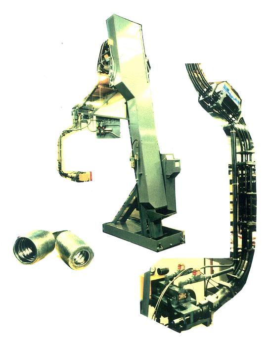
FEED FROM A COLLECTOR HOPPER LOADED FROM THE PREVIOUS OPERATION AT 22" ABOVE THE FLOOR, STEEL HYDRAULIC HOSE COUPLINGS 1 1/2 TO 2 1/2 " DIA. X 1 3/4 TO 2 3/4 LG. THE COUPLINGS WILL BE ORIENTED PIERCED END TRAILING IN TO A SINGLE SLIDING END TO END STREAM TO A POINT 40" ABOVE THE FLOOR, THEN ONE COUPLING AT A TIME WILL BE ESCAPED ROLLING TO A NEST FOR LOADING IN TO MACHINE CELL AT A RATE OF 12 TO 20 PARTS PER. MIN. 6" WIDE ELEVATOR, 1/2 CU. FT. COLLECTOR HOPPER. DWG. PD 8000
