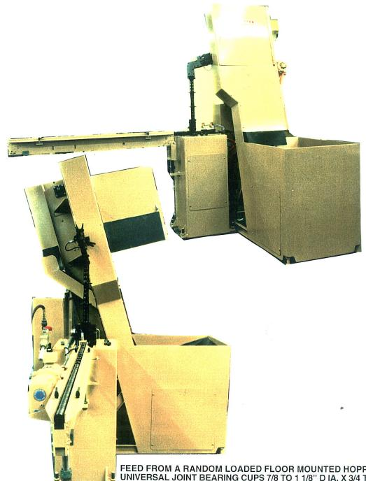
FEED FROM A RANDOM LOADED FLOOR MOUNTED HOPPER, UNIVERSAL JOINT BEARING CUPS 7/8 TO 1 1/8" D IA. X 3/4 TO 1" LG. THE CUPS WILL BE ORIENTED OPEN SIDE OUT ROLLING DIA. TO DIA. TO A VERTICAL 90 DEGREE TWISTED CHUTE TO A PNEUMATIC PUSHER DEVICE ADVANCING ONE CUPAT A TIME TO AN IN PUT CONVEYOR, CONVEYING THE CUPS CLOSED END LOADING IN A CONTINUOUS STREAM TO A CENTERLESS GRINDER AT 42 3/4 ABOVE THE FLOOR AT A RATE OF 1500 TO 2000 PER. HOUR.
