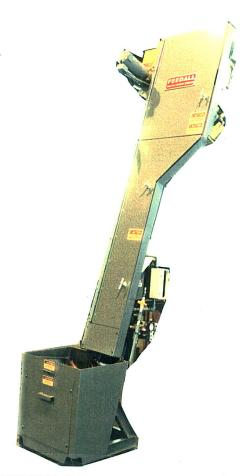
FEED FROM A RANDOM LOADED FLOOR MOUNTED HOPPER TAPERED BEARING ROLLERS .200 TO .625" DIA. X .370 TO .875" LG. THE ROLLERS WILL BE FED END TO END IN A SINGLE CONTINUOUS STREAM TO A POINT 84" ABOVE THE FLOOR TO A CENTERLESS GRINDER ORIENTER (BY CUSTOMER) AT A RATE OF 350 TO 750 PARTS PER. MIN. 4" WIDE ELEVATOR BELT, 1 1/2 CU. FT. HOPPER DWG. P 7745
