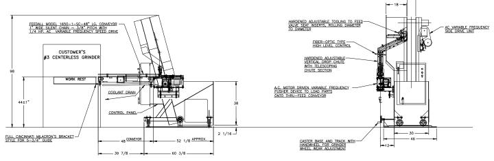
**APPLICATION:** Feed from a random loaded, floor mounted hopper. The Valve Seat Inserts will be oriented in
