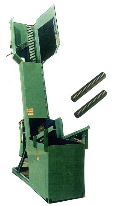
FEED FROM A RANDOM LOADED FLOOR HOPPER PINS .439" DIAMETER BY 2.800 " LONG. THE PINS ARE ELEVATED FROM THE HOPPER THEN ORIENTED END TO END AND FED IN A CONTINOUS STREAM TO A HEIGHT OF 144" ABOVE THE FLOOR TO THE EXISTING CUSTOMER ASSEMBLY MACHINE AT A RATE OF 20 PINS PER. MINUTE. 6" WIDE ELEVATOR BELT, 6 CUBIC FOOT HOPPER. DWG. P 9247 R1
