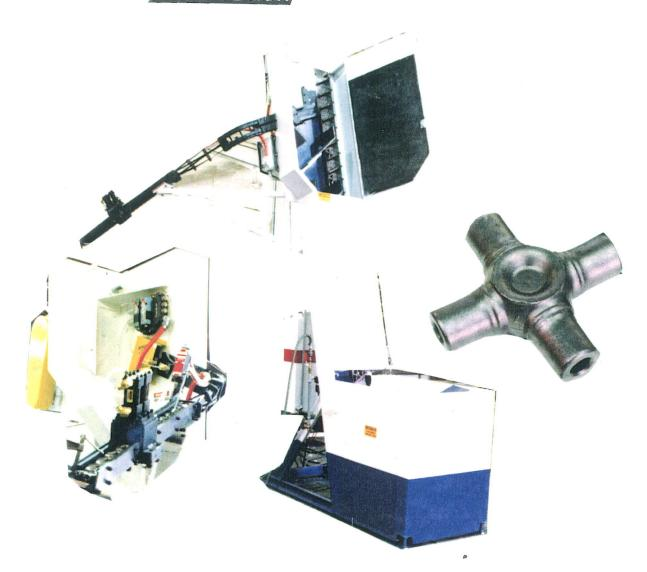
FEED FROM A RANDOM LOADED FLOOR MOUNTED HOPPER, AUTO UNIVERSAL SPIDERS. THE SPIDERS MUST BE ORIENTED LAYING FLAT IN A SINGLE STREAM, THEN ESCAPED ONE AT A TIME TO A HORIZONTAL LOCATION 77 1/2" ABOVE THE FLOOR AT A RATE OF 300 PER. HOUR. DWG. PD 9043 R 1
