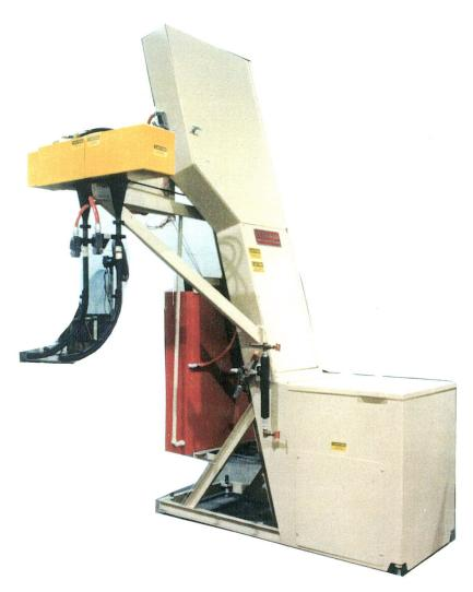
FEED FROM A RANDOM LOADED FLOOR MOUNTED HOPPER, POWER STEERING IN PUT SHAFTS. THE SHAFTS WILL BE ELEVATED FROM THE HOPPER THEN FED END TO END AND ORIENTED SMALL DIA. END LEADING AND FED IN TO TWO INDEPENDENTLY SATISFIED VERTICAL CHUTES TO A HORIZONTAL POSITION, 10 1/2" APART, 45" ABOVE THE FLOOR AT A RATE OF TWO PARTS EVERY 15 SECONDS, FOR LOADING IN TO DIAL FOR A REAMING MACHINE. 7 1/2" WIDE ELEVATOR BELT, 6 CU. FT. HOPPER DWG. PD 8210 R 1
