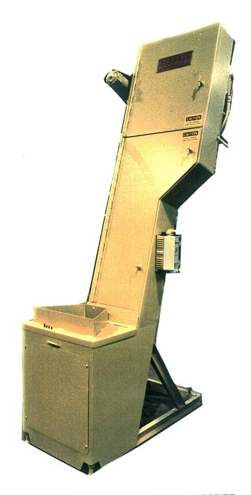
FEED FROM A RANDOM LOADED FLOOR MOUNTED HOPPER, TAPERED BEARING ROLLERS, .200 TO .625" DIA. THE ROLLERS ARE TO BE ORIENTED END TO END IN A SINGLE END TO END STREAM TO A POINT 76" ABOVE THE FLOOR AT A RATE OF 350 TO 700 PER. MIN. TO A CENTERLESS GRINDER. 4" WIDE ELEVATOR BELT, 3 CU. FT. HOPPER. DWG. P 7409 R 3
