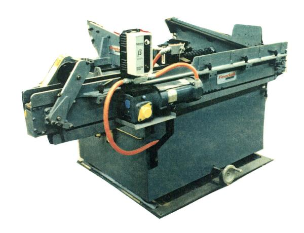
FEED FROM A MANUALLY LOADED SINGLE ROW MAGAZINE STEEL SHAFTS 1 15/16 TO 4" DIA. X 12 TO 36" LG. THE SHAFTS WILL BE ESCAPED ONE AT A TIME TO THE FRONT MOUNTED CROSS CONVEYOR THEN FED END TO END TO A CENTERLESS GRINDER AT 40" ABOVE THE FLOOR. DWG. PD 8484
