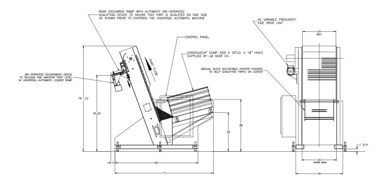
**APPLICATION:** Feed from an automatic or hand loaded, floor-mounted hopper. Steel Bars will be elevated
