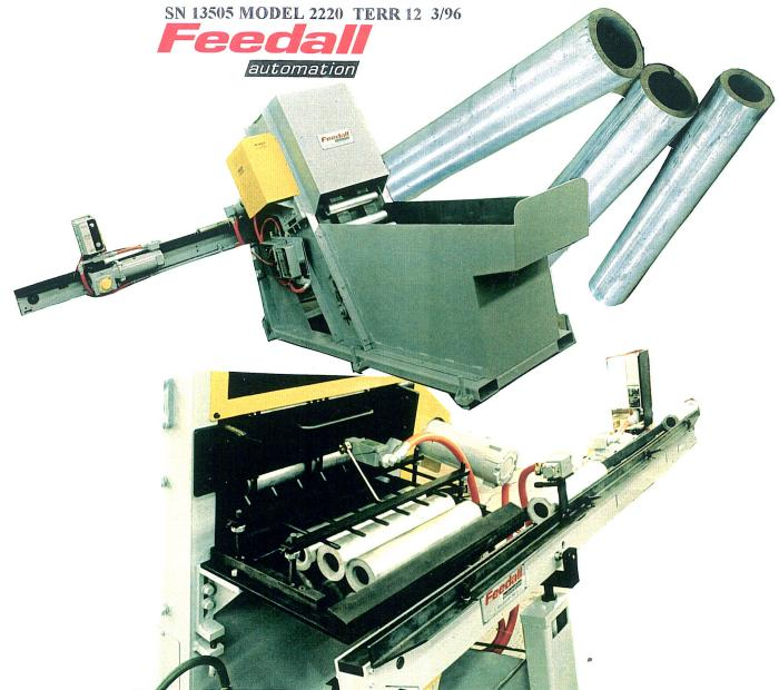
FEED FROM FLOOR HOPPER ALUMINUM TUBES
