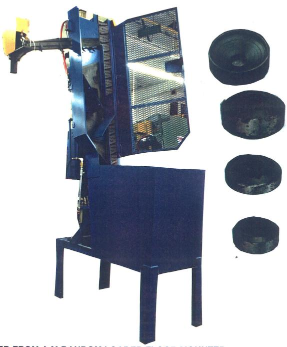
FEED FROM A M RANDOM LOADER FLOOR MOUNTED HOPPER, FORGED STEEL PREFORMS. THE PARTS WILL BE FIRST ORIENTED ROLLING DIAMETER TO DIAMETER THEN FED AND ORIENTED COUNTER BORE FACE UP IN TO A VERTICAL STACK AT 72" ABOVE THE FLOOR AT A RATE OF 30 PER. MIN.
