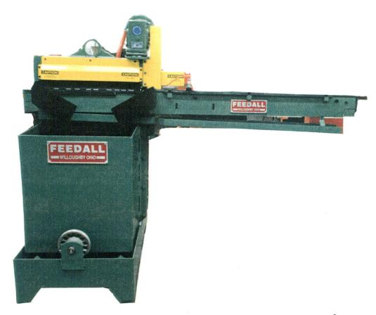
FEED FROM A MANUALLY STACKED OR RANDOM LOADED FLOOR MOUNTED HOPPER ARMATURE SHAFTS .320 TO .381" DIA. X 2 TO 8" LG. THE SHAFTS WILL BE ELEVATED THEN DESCHARDED ROLLING ONTO THE CROSS CONVEYOR THEN FED END TO END IN A CONTINUOUS STREAM TO A CENTERLESS GRINDER AT 42 3/4" ABOVE THE FLOOR AT A RATE OF 200" PER.MIN.
