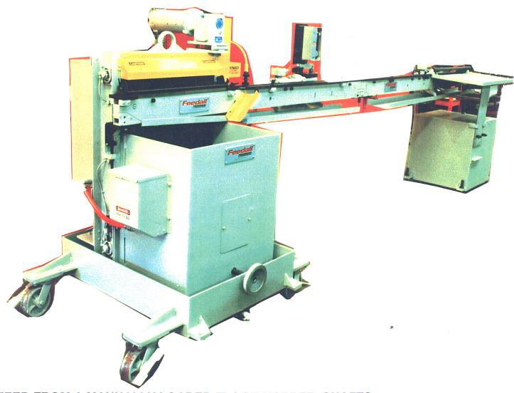
FEED FROM A MANUALLY LOADED FLOOR HOPPER, SHAFTS .400 TO .600" DIA. TO 23" LG. THE SHAFTS WILL BE ELEVATED FROM THE HOPPER THEN DISCHARGED ROLLING TO THE FRONT MOUNTED CROSS CONVEYOR THEN FED END TO END TO A CENTERLESS GRINDER AT 42" ABOVE THE FLOOR AT A RATE OF 75 TO 150" PER. MIN. THE SHAFTS WILL THEN EXIT THE GRINDER AND BE CONVEYED 72" THEN DISCHARGED ROLLING TO A COLLECTION TRAY FOR MANUAL INSPECTION AND UN- LOADING.
