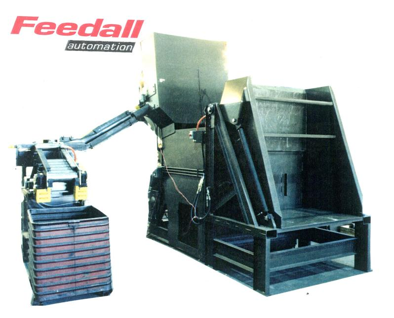
FEED FROM A RANDOM LOADED FLOOR MOUNTED HOPPER, STEEL BILLETS 3 1/2 TO 5" DIA. X 5 TO 13" LG. THE BILLETS WILL BE ELEVATED AND ORIENTED IN A SINGLE END TO END STREAM THEN TRANSFERRED ROLLING DIAMETER TO DIAMETER INTO A MAGAZINE. THE BILLETS WILL THEN BE ESCAPED ONE AT A TIME TO THE CUSTOMERS PUSHER DEVICE AT 48" ABOVE THE FLOOR AT A RATE OF 100 TO 400 PER. HOUR.
