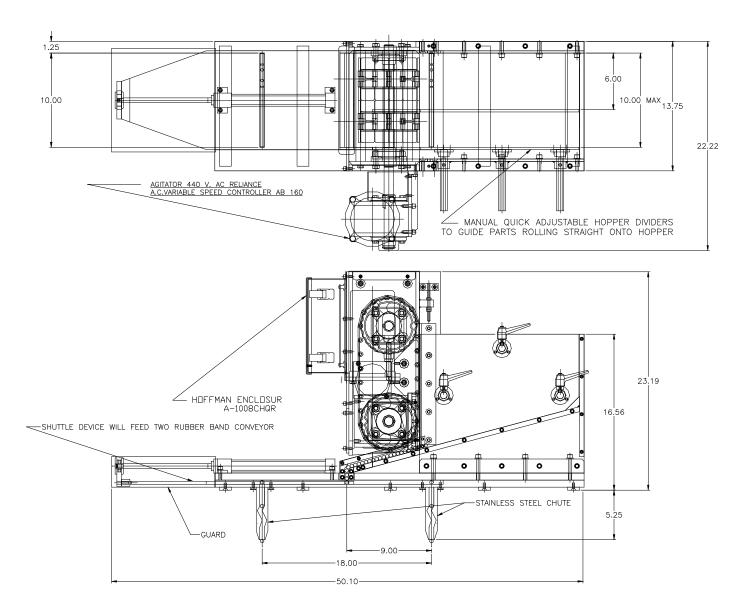
**APPLICATION:** Feed from a manually loaded magazine, Throttle Body Shafts will be agitated within the
