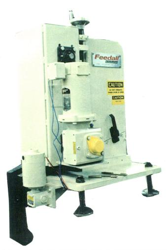
FEED FROM A MANUALLY LOADED MAGAZINE THROTTLE BODY SHAFTS .392" DIA. X 5.67 " LG. THE SHAFTS WILL BE FED ROLLING DIAMETER TO DIAMETER IN TO A RADIAL ORIENTING EACH SHAFT BY THE MILLED FLATS FOR THE THROTTLE PLATES, VERTICAL. THE SHAFTS WILL BE DISCHARGED IN A VERTICAL STACK FOR PICK UP FROM THE ASSEMBLY MACHINE AT RATE OF 12 TO 15 PER. MIN. DWG. P 8453
