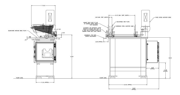
**APPLICATION:** Feed bars from a manually loaded, floor mounted magazine. Steel Tubes will be fed in a
