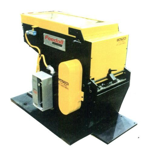
FEED FROM A MANUALLY LOADED MAGAZINE AUTOMOTIVE WATER PUMP SHAFTS .500 TO .800" DIA. X 4 TO 8" LG. THE SHAFTS WILL BE ESCAPED ROLLING ONE AT A TIME TO THE GRINDER LOAD STATION AT A RATE OF 240 PER. HOUR. DWG. PD 8973 R 2
