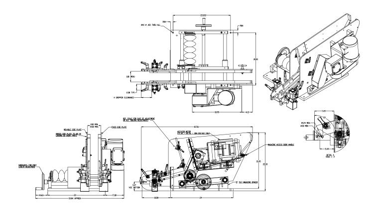
**APPLICATION:** Feed Steel Bars from a manually loaded, floor mounted magazine. Bars will be fed in a
