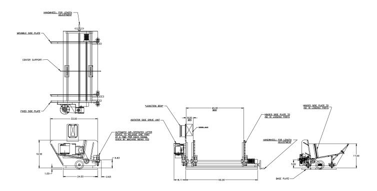
**APPLICATION:** Feed bars from a manually loaded, floor mounted magazine. Then will be fed in a continuous
