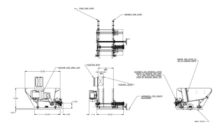
**APPLICATION:** Feed bars from a manually loaded, floor mounted magazine. Then will be fed in a continuous
