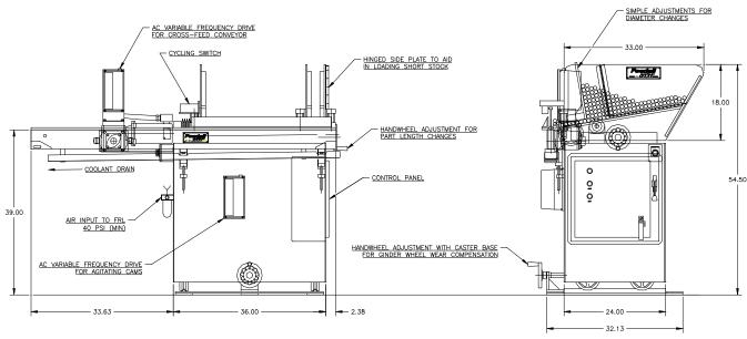
**APPLICATION:** Feed from a manually loaded, floor mounted magazine. Shafts will be fed in a continuous
