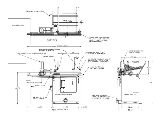
APPLICATION: Feed Piston Rods from a manually loaded, floor mounted magazine. The rods will be fed in a
