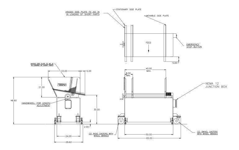
**APPLICATION:** Feed from a manually loaded, floor mounted magazine. The Steel Tubes will be fed in a
