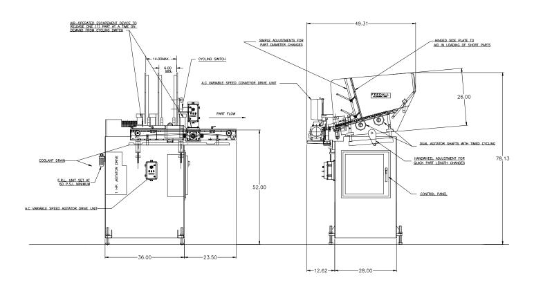
**APPLICATION:** Feed from a manually loaded, floor mounted magazine. The Sheared Steel Bars will be
