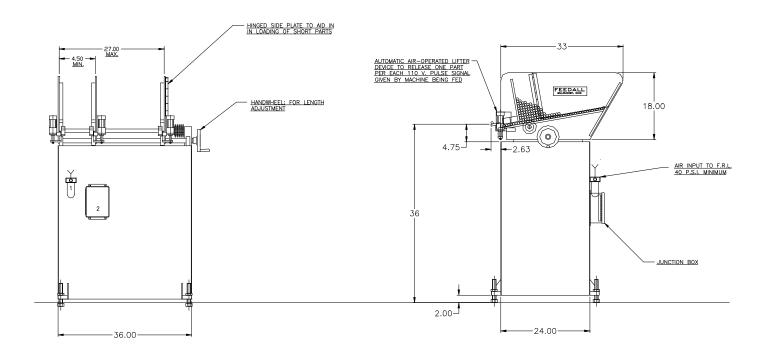
**APPLICATION:** Feed from a manually loaded floor mounted magazine. The Steel Shafts will be discharged one at a time relling diameter for each signal given by the Breach Machine.
