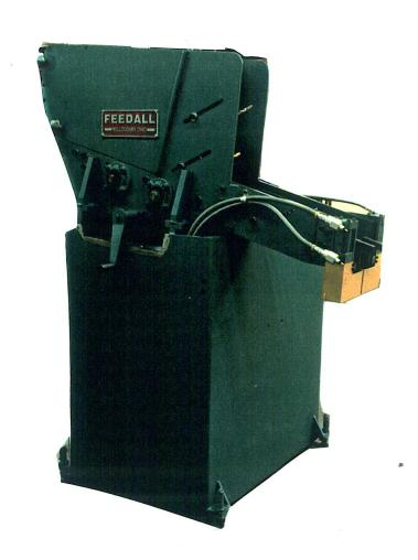
FEED FROM A MANUALLY LOADED MAGAZINE STEEL SHEAR CUT BARS, 3/4 TO 2" DIA.X 6 TO 22" LG. THE BARS WILL BE ESCAPED ROLLING ONE AT A TIME TO AN INDUCTION COIL AT 42" ABOVE THE FLOOR AT A RATE OF 10 TO 20 PER. MIN. DWG. PD 7474
