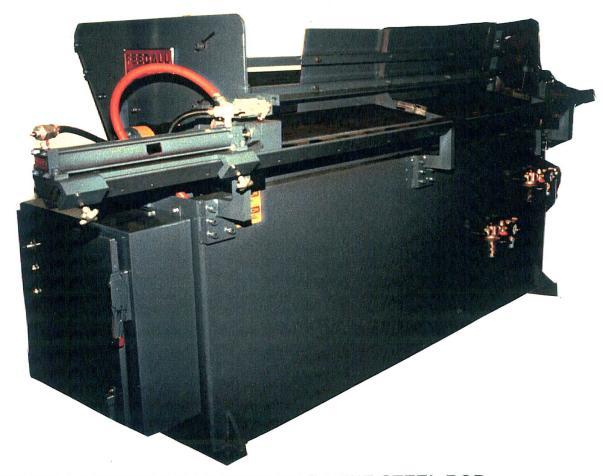
FEED FROM A MANUALLY LOADED MAGAZINE STEEL ROD BLANKS FOR THREADED RODS 1/4 TO 1" DIA. X 12 TO 72" LG. THE BLANKS WILL BE ESCAPED ROLLING ONE AT A TIME TO THE FRONT MOUNTED PNEUMATIC PUSHER THEN ADVANCED TO THE THREAD ROLLER AT A RATE OF 10 TO 20 PER. MIN. AT A HEIGHT OF 42" ABOVE THE FLOOR. DWG. PD 7133 R 2
