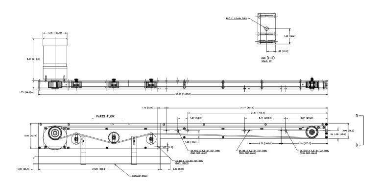
**APPLICATION:** Convey Fastener Blanks from the workrest of a LANDIS Viking Centerless Grinder. The parts
