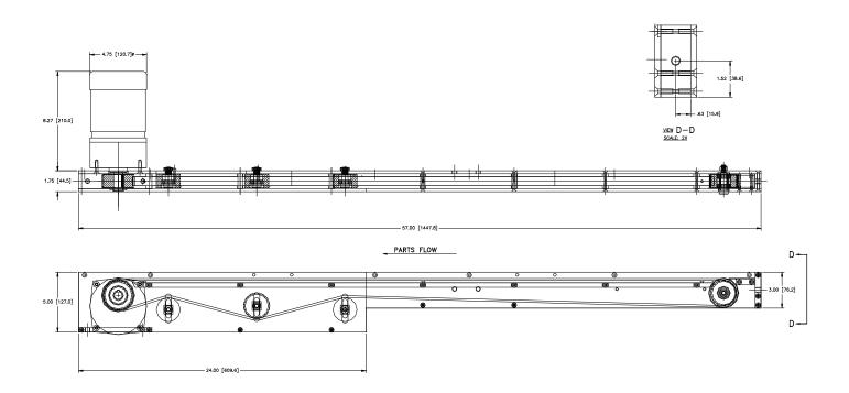
**APPLICATION:** Convey Shoulder Pins from a CINCINNATI Viking Centerless Grinder. The shafts will exit
