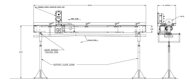
**APPLICATION:** Convey Steel Shafts to the workrest of a CINCINNATI Centerless Grinder.
