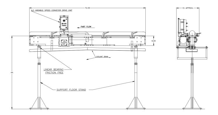
**APPLICATION:** Convey Steel Pins between the workrests of two CINCINNATI #2 EA Centerless Grinders.
