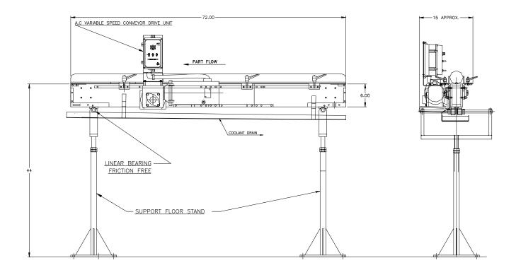
**APPLICATION:** Convey Steel Pins from the workrest of a CINCINNATI #2 EA Centerless Grinder.
