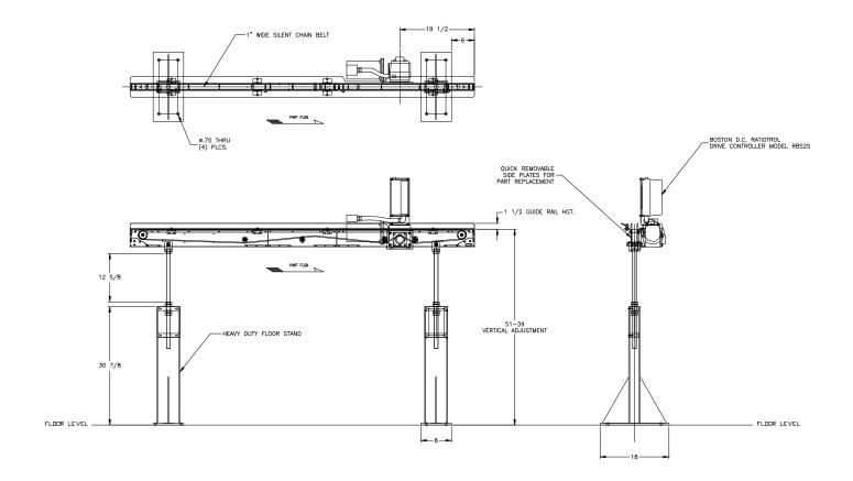
**APPLICATION:** Accept Suspension Bushing Inner Metal Tubes and convey them to a Storage Tub.
