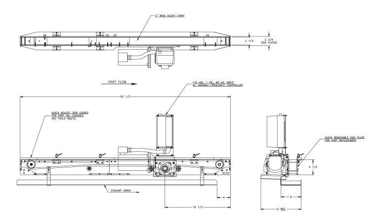
**APPLICATION:** Convey Motor Rotors to the workrest of a Centerless Grinder.
