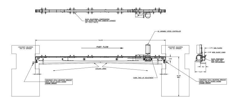
**APPLICATION:** Convey Steel Tubes between the workrests of two CINCINNATI Model 340-20 Centerless
