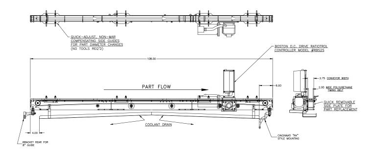
**APPLICATION:** Convey Rocker Arm Shafts between workrests of two Centerless Grinders.
