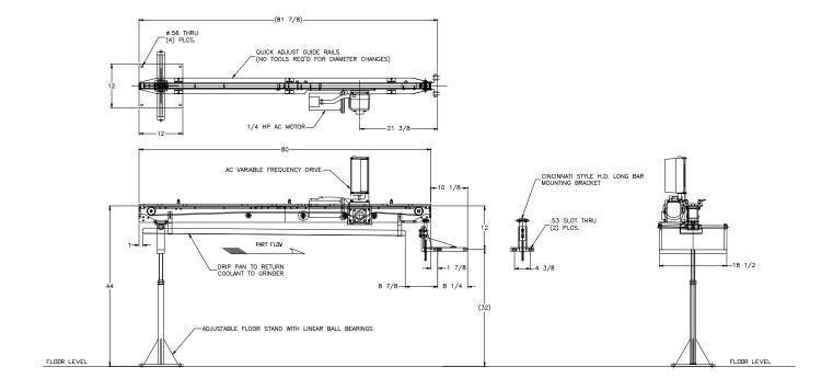
APPLICATION: Convey steering rack blanks to and from the workrest of a CINCINNATI model 350-20 AE
