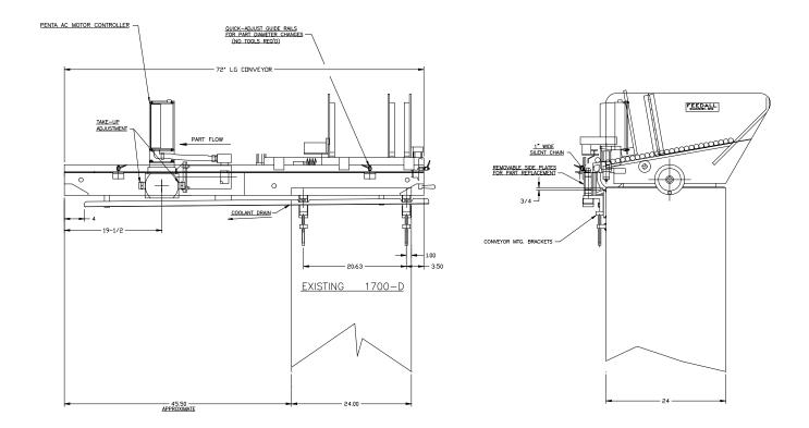
**APPLICATION:** Convey Steel Bars to the workrest of a Thread Roller.
