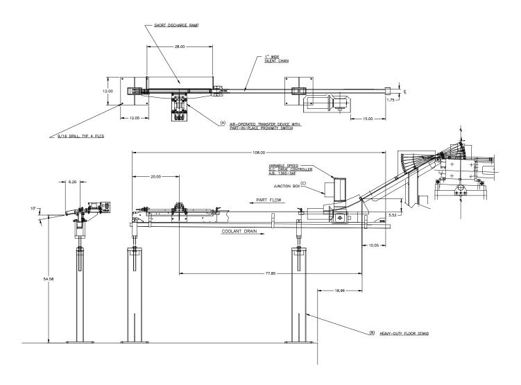
**APPLICATION:** Convey Steering Racks from Detroit Broach to a Parts Washer. The parts will exit the
