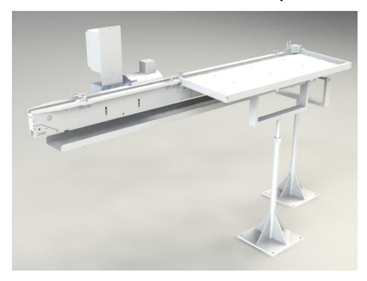
APPLICATION: Convey Steering Racks (25mm-32mmØ x 400mm-900mm Lg.) from workrest of a
