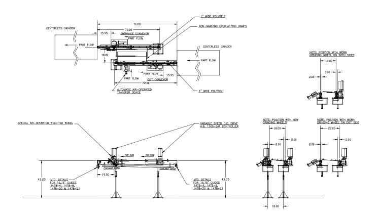
**APPLICATION:** Convey Steering Racks from the workrest of a Centerless Grinder to the workrest of another
