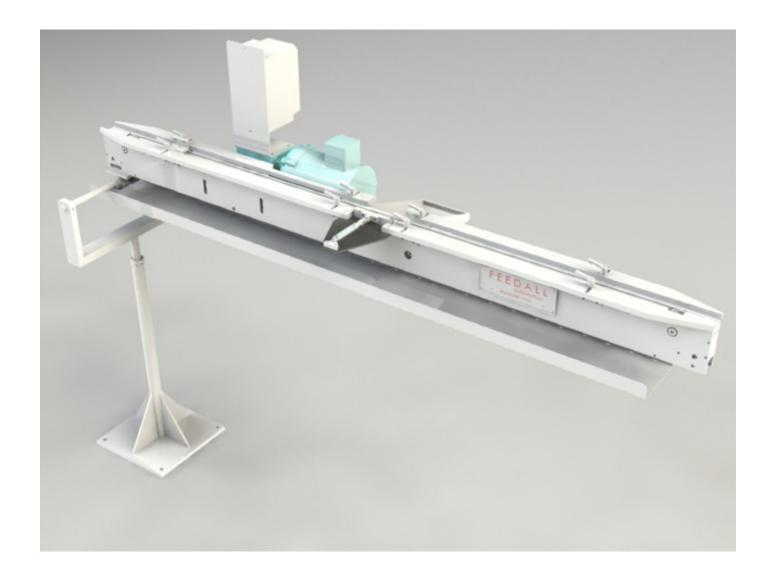
**APPLICATION:** Convey Universal Joint Bearing Cups from the workrest of a CINCINNATI Model 340-20
